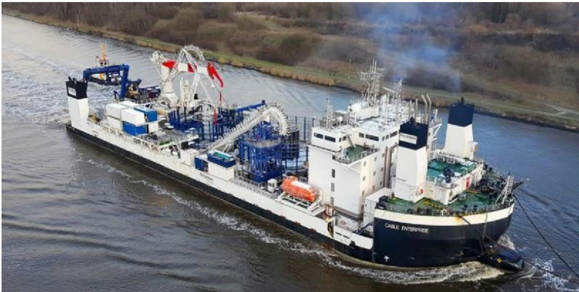
Figure 3.6: Example of a primary Cable Laying Barge [approximate size 125m (l) x 32m (b)]
