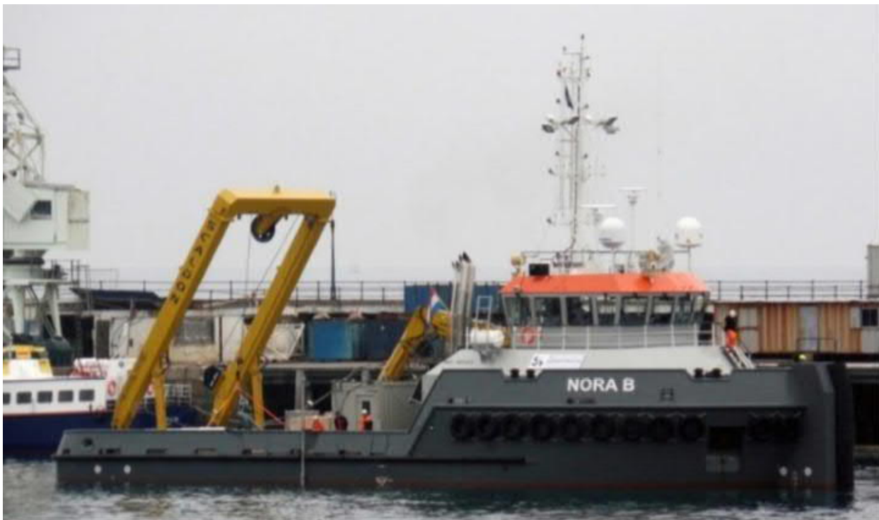
Figure 3.8: Example of a Pre-Lay Grapnel launch vessel
