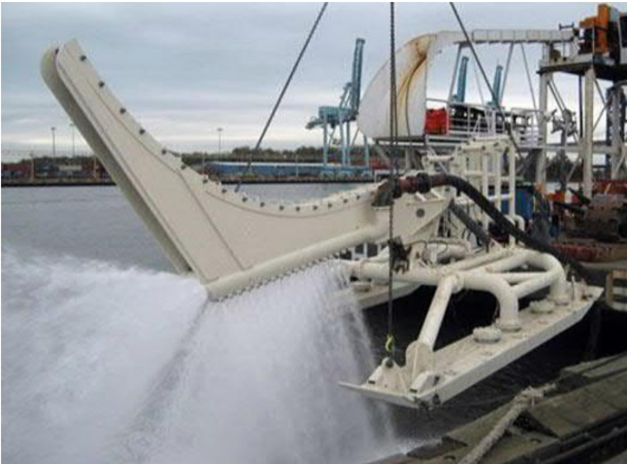
Figure 3.10: An example of a jetting tool
